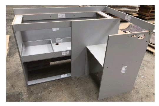
Each campervan needed cabinetry for the kitchenette to house the sink including storage underneath, plus cabinets for the microwave and small fridge, and two long bed units with storage compartments.
